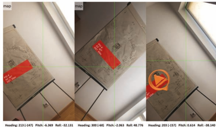
Figure 11. Test application presenting labels and 3D models of spatial objects based on sensor readings.
