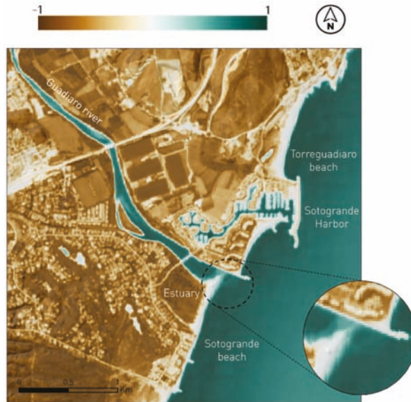
Figure 6. Total climatography (2017–2020) using Sentinel-2 L2A images and NDWI index for the Guadiaro river mouth. Scale 1:15,000.
