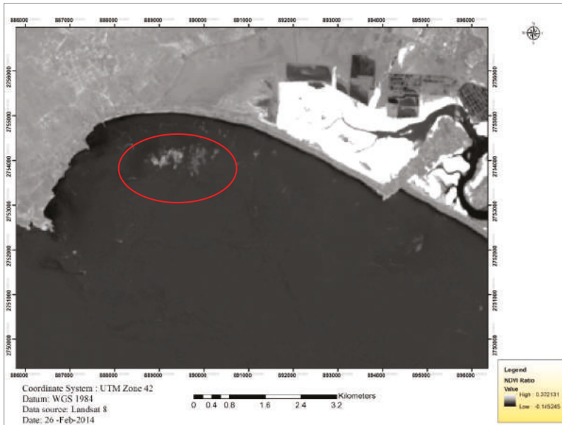
Figure 4. This figure shows NDVI with values ranging from -0.145 to 0.372 . The red oval highlights the seaweed patches (26 February 2014).
