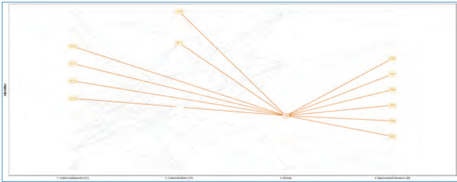
Figure 20.8. The Flexible Resilience Analysis Template (FRAT) Shiny app will display the connections between the system components, system functions, and threats. In this example, the T2 threat (data exfiltration) is highlighted. It has connections to different system components such as workstations and servers, and the business applications. It also connects to two system functions: L3 connectivity and security functions and policies. Improvement measures related to this threat include training, governance, and alerts.
