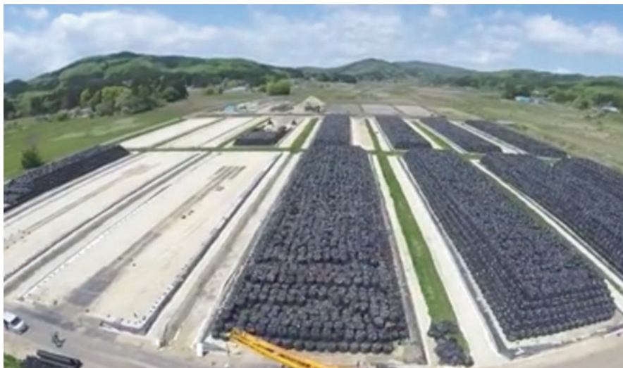
Photo 16.1 Contaminated soil bags piled up in a temporary-temporary storage place (Resurrection of Fukushima 2017). (Photo and video provided: NPO Resurrection of Fukushima)
